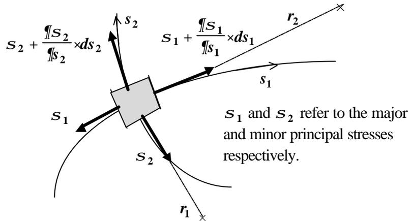
Figure 1: Principal stress components using curvilinear coordinates.
