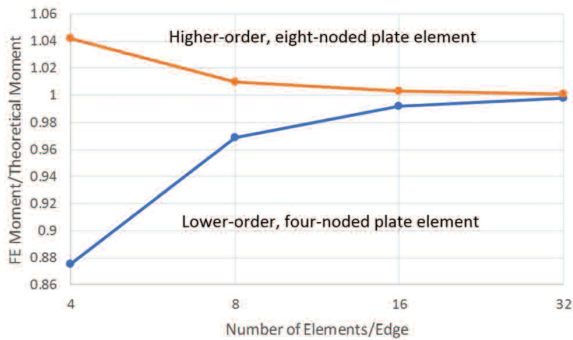
Figure 8: Convergence of bending moment for lower and higher-order plate elements
