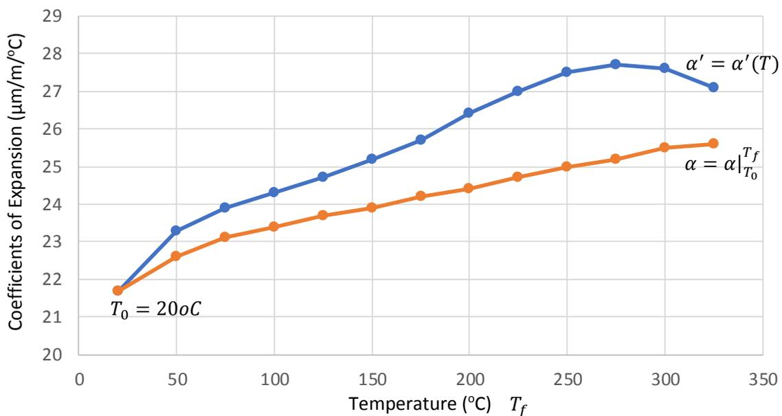
(b) Coefficients of expansion as functions of temperature
