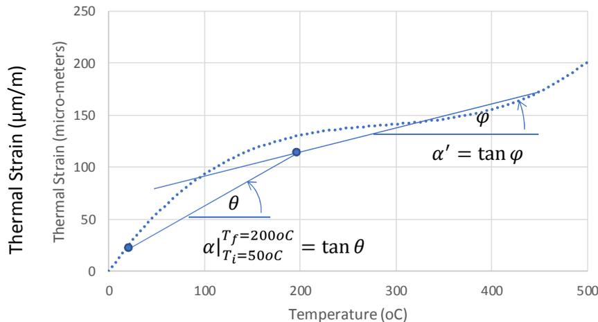
Figure 1: Coefficients of expansion vs Temperature (°C)
