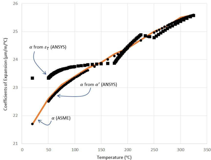
**Figure 4:** Mean coefficient of expansion from ANSYS
