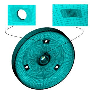
The hole in the web leads to a stress concentration factor of about 2 whereas the hole in the hub, used as a grease hole to lubricate the bearings, leads to a stress concentration of about 2.5.
