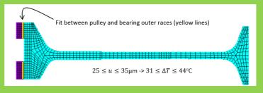
The interference was induced by applying an appropriate temperature decrease to the pulley. The radial force between bearings and pulley was established at the current speed and at the proposed increased speed and with the coefficient of friction the limiting torque for the fit was determined.
