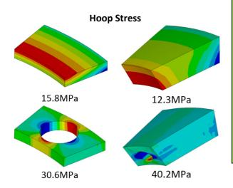
With the increase in speed for the new machine it is necessary to assess the interference fit. This assessment was undertaken using axisymmetric FE analysis which now included the outer races of the bearings with contact elements between the components.
