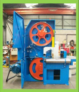
The manufacturer is designing a new machine to run at a higher speed and requested RMA's assistance in undertaking a finite element stress analysis of the pulleys in order to establish whether the existing cast iron would be acceptable to take the higher stresses.
