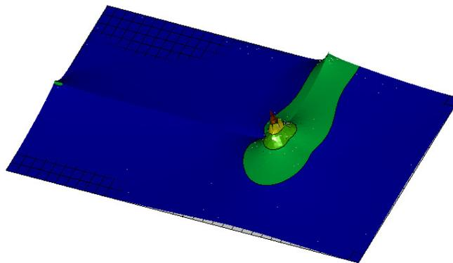
**Figure 4:** Maximum principal bending moment contours (elastic)
