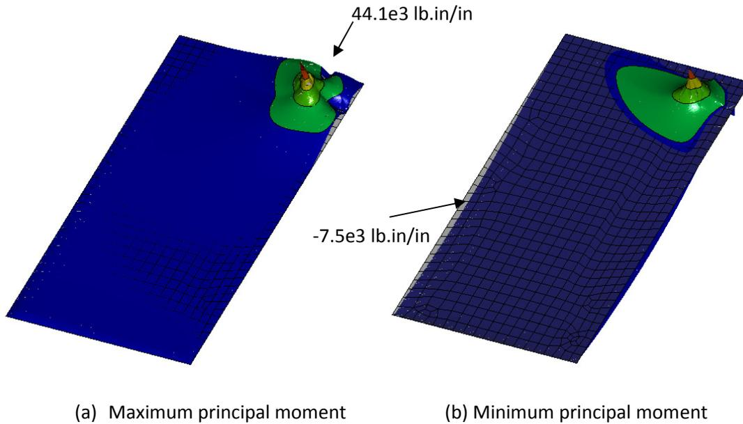
**Figure 14:** Principal bending moment contours (elastic)
