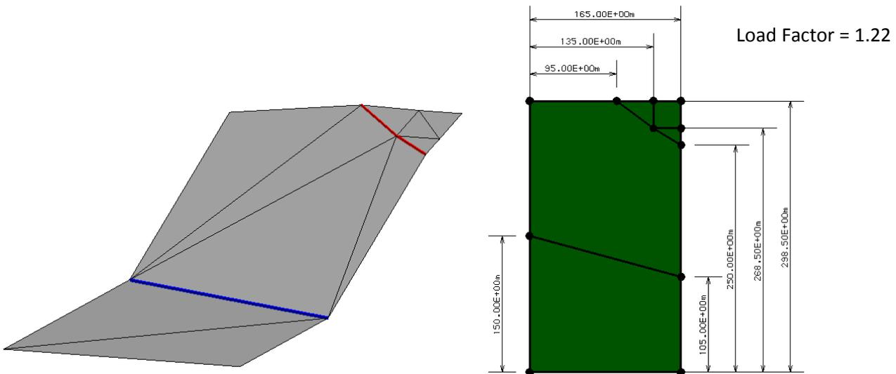
**Figure 17:** Yield line pattern on deflected shape and optimal positions of points
