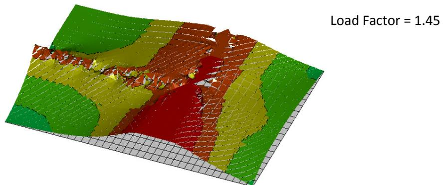
**Figure 7:** Maximum principal bending moment contours (equilibrium limit - Bottom = Top Steel)
