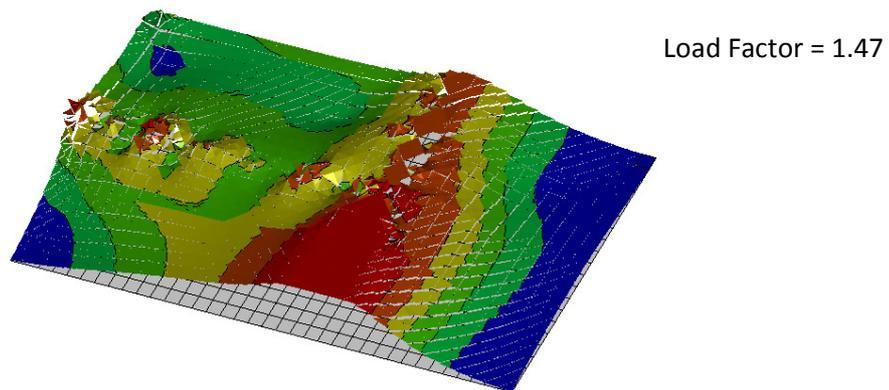
**Figure 9:** Maximum principal bending moment contours (equilibrium limit - Bottom = 0.1xTop Steel)
