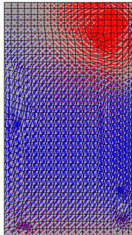
**Figure 15:** Principal bending vectors (elastic)
