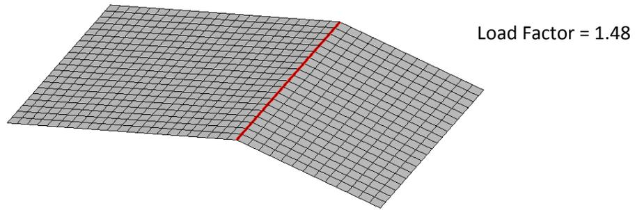
**Figure 6:** Yield line pattern and deflected shape (Top and bottom steel identical)
