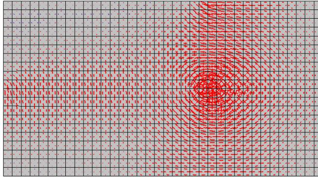
**Figure 5:** Principal bending vectors (elastic)
