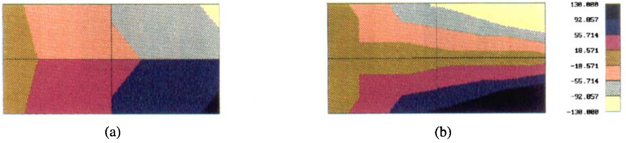
Plate 1. Contours of the \tau_{xy} -component of stress for Mesh 1 of Problem 1: (a) conforming (4-noded) element; (b) equilibrium (linear) element
