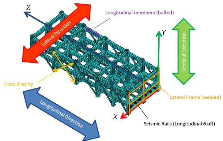
A finite element analysis of the structure is generally conducted to establish member stress resultants, shear force and moment distributions for the structural model considered here. There is essentially three approaches that may be adopted:
