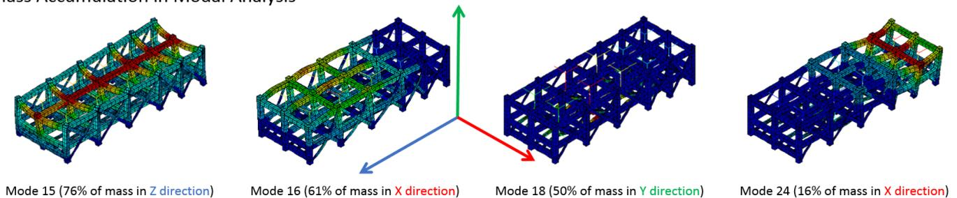
Having produced a verified set of member forces and moments these were then used in an EC3 code assessment with unit partial factors on both material and loading. The utilisation ratios for the different types of structural members were calculated and found to be less than 1/3 for the RSA. With the ESM the utilisations were significantly greater, as expected from the conservative nature of this approach, but still less than unity.
