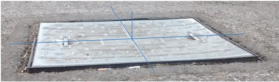
Figure 9: Permanent and large deflections of a plate
